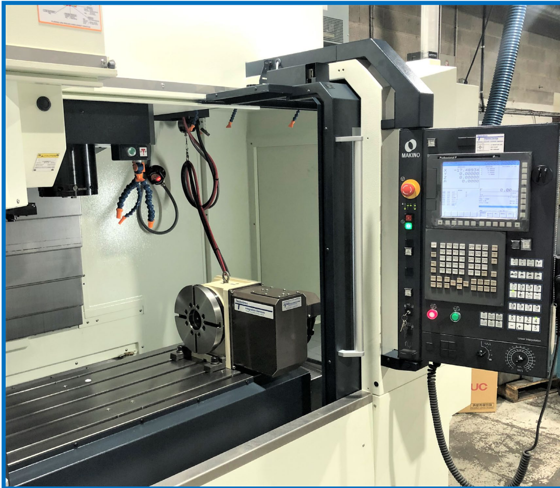
Tsudakoma RWA-250R, M 4 th axis installation on a Makino PS105 (VMC) with the PRO P control
