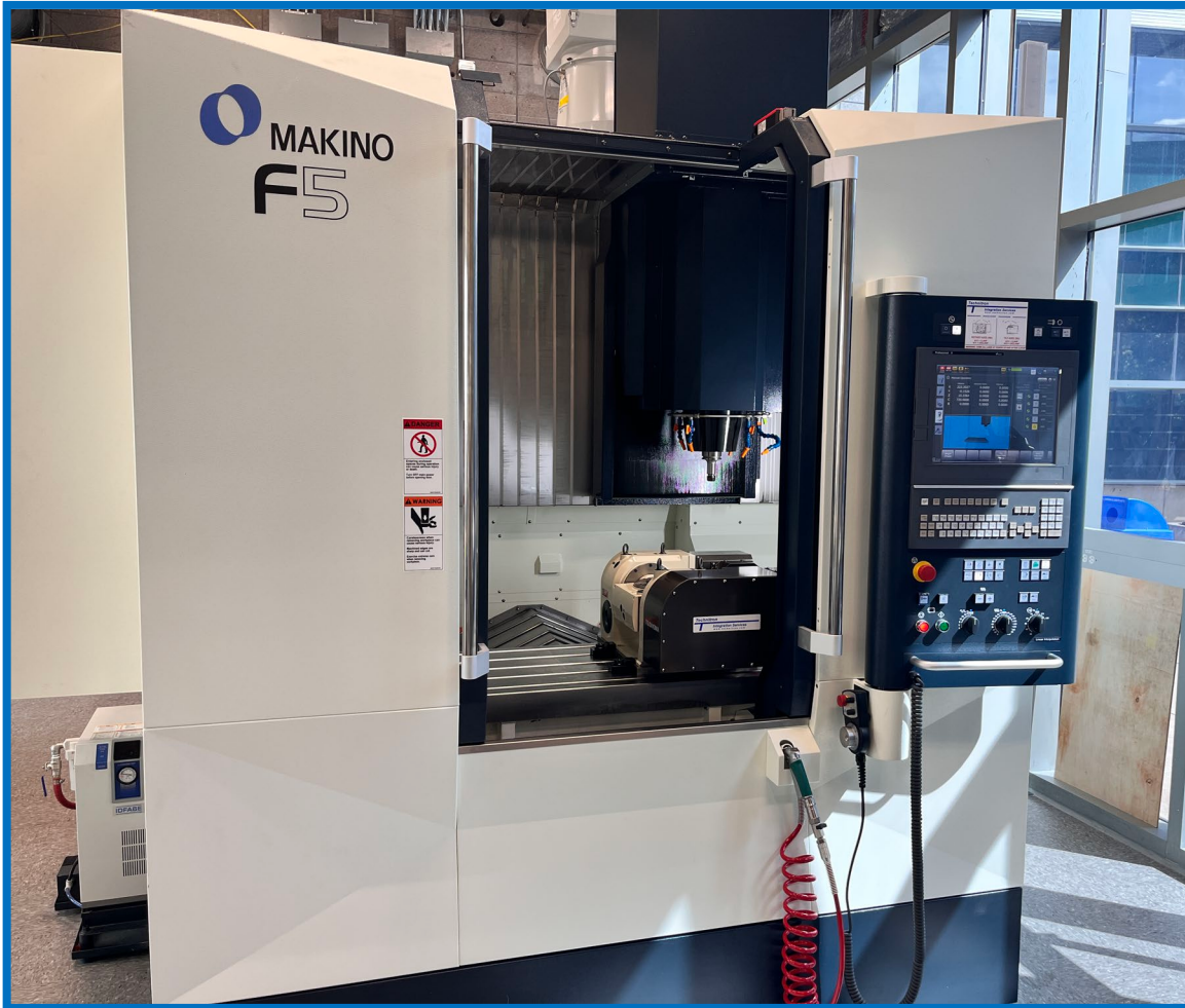
Tsudakoma TWA-160, M - 4 th / 5 th axis installation on a Makino F5 (VMC) with the PRO 6 control
