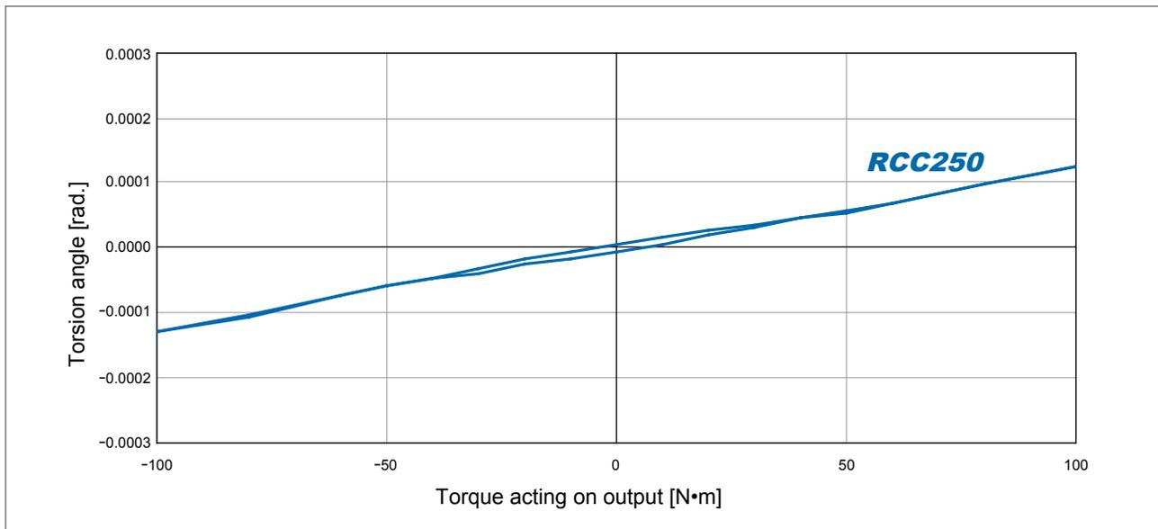
For a general reducer, the hysteresis graph can be obtained by applying torque to the output shaft, and plotting the generated torsion angle.
