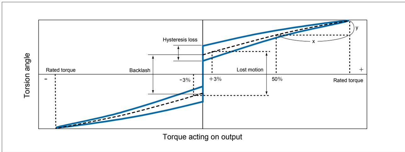
**Backlash** Rotation angle which can arise even with zero torque (looseness)
