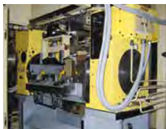
Synchronizers movement of 2 off CNC401T Tubular roller bearing is installed against the thrust load. Therefore, when 2 rotary tables are faced on both side to synchronise movement, the system can be run without affecting the heat expansion of the rotary table.
